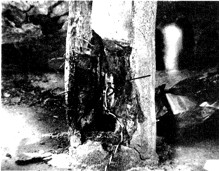
f) Strain Gage - East/West Bending on Embedded Steel
