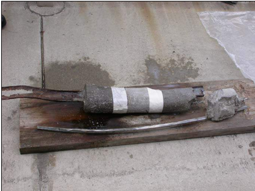
Figure 22: Samples of mortar and reinforcing previously removed from towers used for testing application of water repellent and penetrating rust inhibitor before treatment.
