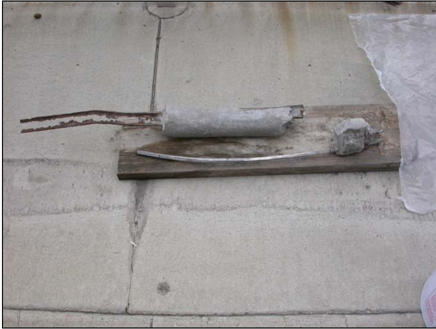
Figure 22: Samples of mortar and reinforcing previously removed from towers used for testing application of water repellent and penetrating rust inhibitor before treatment.
