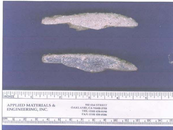
Photo 2. Sample 1 cross-sectional slices. The bottom section was treated with a pH indicator solution. The purple color of the paste indicates a pH greater than 13 (non-carbonated paste).
