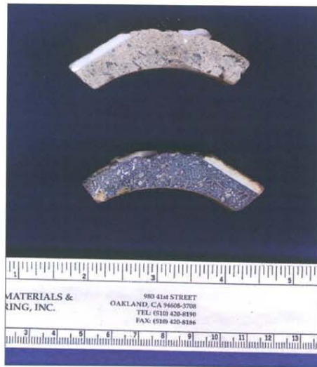
Photo 4. Sample 3 cross-sectional slices. The bottom section was treated with a pH indicator solution. The purple color of the paste indicates a pH greater than 13 (non-carbonated paste).
