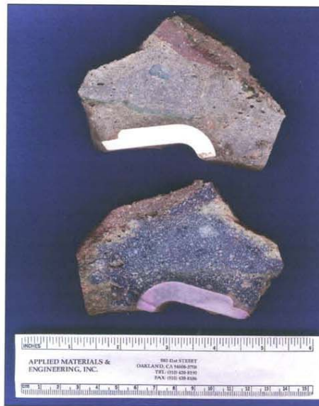
Photo 5. Sample 4 cross-sectional slices. The bottom section was treated with a pH indicator solution. The purple color of the paste indicates a pH greater than 13 (non-carbonated paste).
