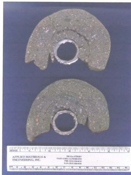
Photo 3. Sample 2 cross-sectional slices. The bottom section was treated with a pH indicator solution. The paste changed from yellow to green in color, indicating the entire thickness had a pH of less than 10 (carbonated paste).
