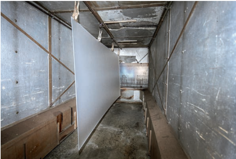
1 A four-by-eight-foot sheet of imported acrylic, with a special velvety finish, is hung from clamps and heated to approximately four hundred degrees Fahrenheit in a custom-made, walk-in oven.
