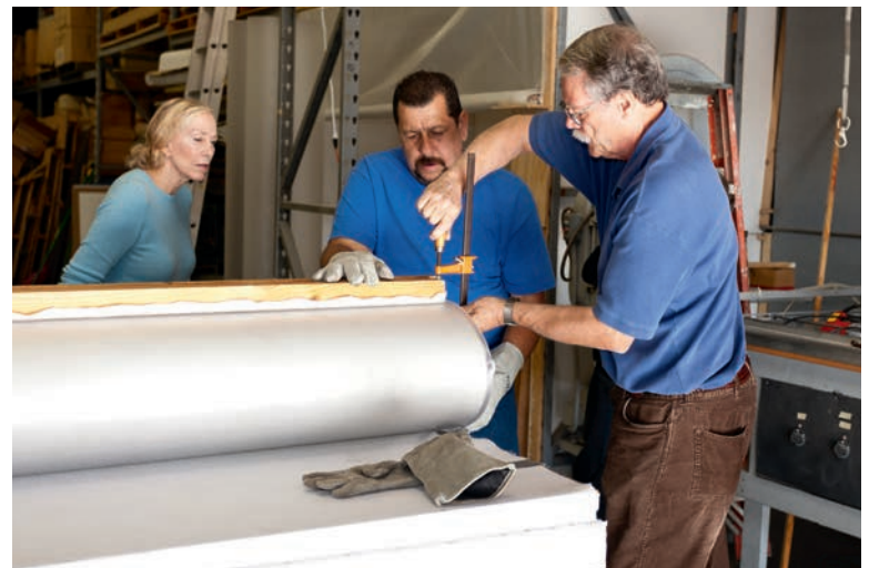
4 Willis, under the artist's watchful eye, clamps the hot acrylic in place to assure a perfectly formed column. It is crucial that the surface of the molded acrylic form be pristine and blemish-free.
