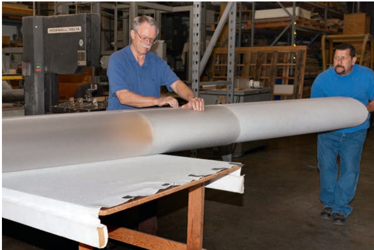
5 Once the acrylic has cooled, the mold is carefully removed. The same mold will be reused to fabricate additional columnar elements for Pashgian's sculptural installation.
