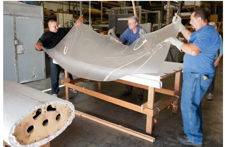
2 The hot, pliable sheet of acrylic is removed from the oven and placed on a nearby foam-covered table by Albert Leal and Robert Castañeda, under the supervision of fabricator Lance L. Willis.
