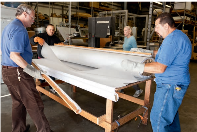
3 Pashgian watches in the background as Leal and Castañeda wrap the softened acrylic around a custom-made, foam-covered wood mold, while Willis stands in the foreground with a specially fashioned tool that he will use to insure a bubble-free surface on the molded acrylic. The entire wrapping and smoothing process must happen very quickly, before the acrylic cools to the point that it loses its pliability.
