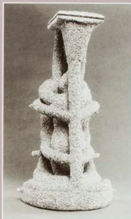
7 A finely granulated ceramic is gradually applied to the surface of the model and its conduits until it becomes thick and coarse. The end result is called an "investment mold." The mold is then dried and heated; the wax melts and flows out of the mold, leaving a space between the fire resistant clay model and the investment mold. This process is called the "lost-wax method."
