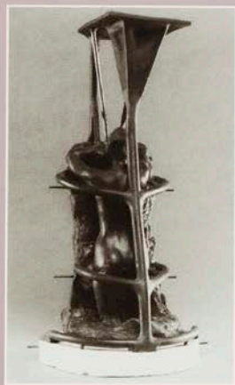
6 Wax conduits, called sprues and gates, are attached to the model. They act as channels through which the wax, when heated, will escape.
